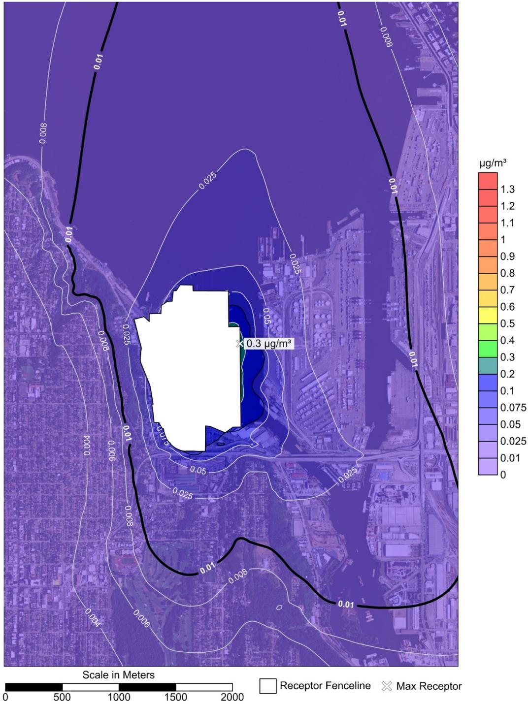
**Figure 6. Alternative 3 (2030): Model-Calculated Diesel Particulate Concentrations Attributable to Terminal 5 Activities**
