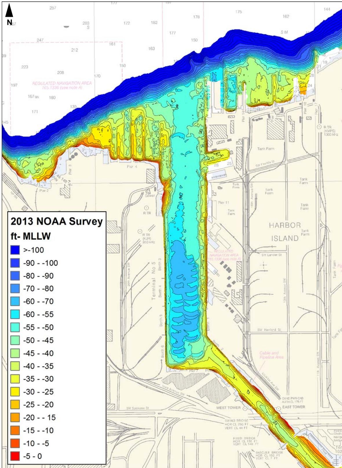
Figure 3: NOAA 2013 Bathymetry of the Duwamish River – West Waterway
