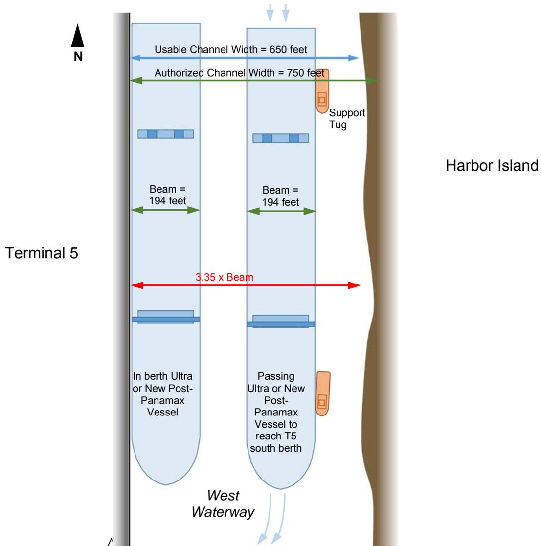
**Figure 15: Scenario 2 Berthing Separation Distance Using Navy/ROM Evaluation Method**
