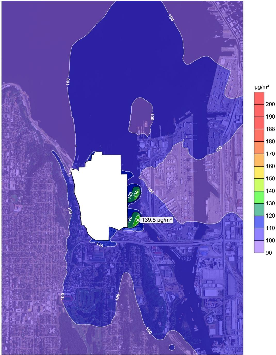
**Figure 4. Alternative 3 (2030): Model-Calculated 1-Hour NO<sub>2</sub> Concentrations**
