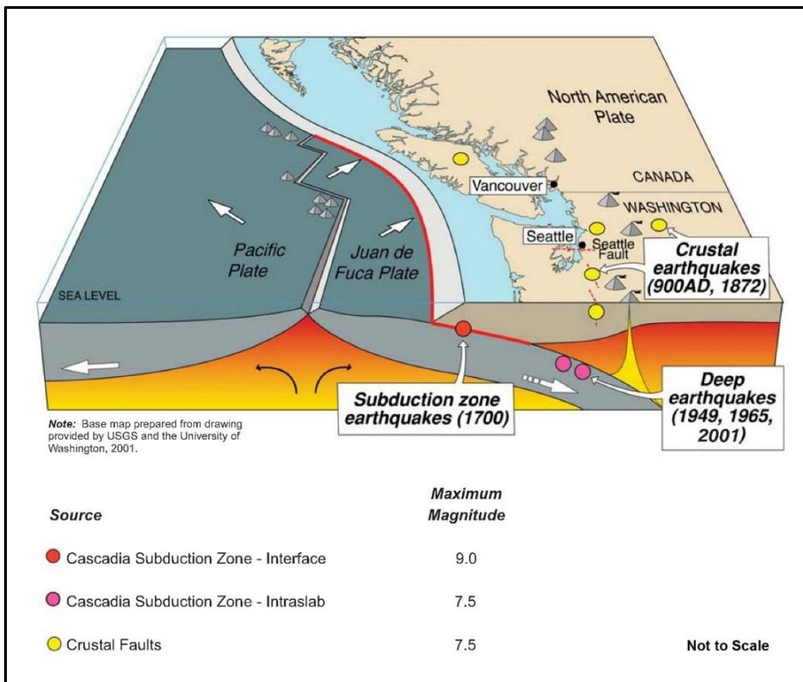
Figure 4. Cascadia Subduction Zone Earthquake Sources
