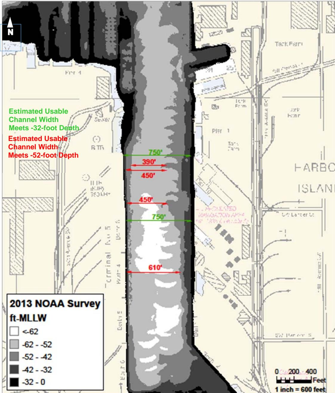
Figure 16: Location Used in Channel Width Analysis (NOAA 2013)
