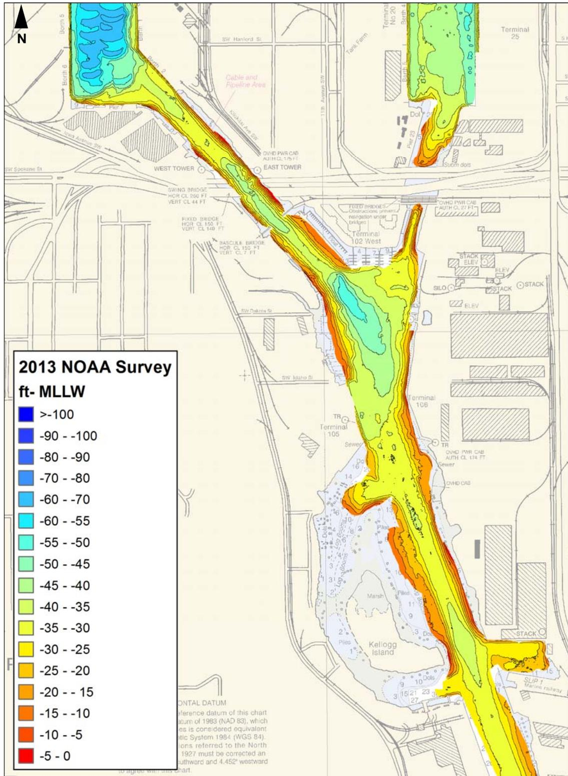
**Figure 4: NOAA 2013 Bathymetry of the Duwamish River – West Waterway to Lower Duwamish Waterway**
