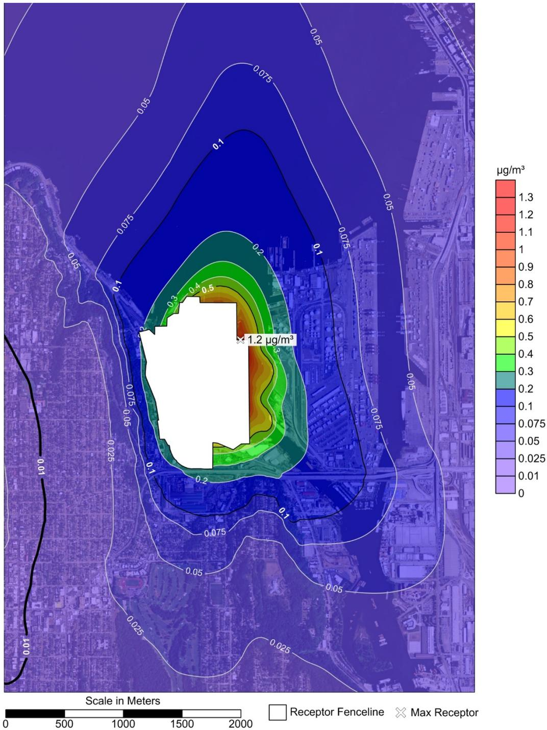
**Figure 5. Alternative 1 (2020): Model-Calculated Diesel Particulate Concentrations Attributable to Terminal 5 Activities**
